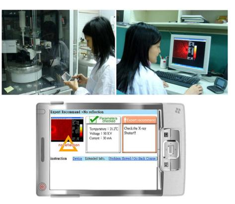
Fig. 4. Illustrative example of guiding the researcher to operate the X-ray diffractometer and the structural analysis software.
